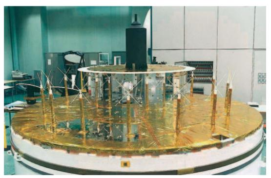
Figure 1. The flight-model MCP Antenna Subsystem
