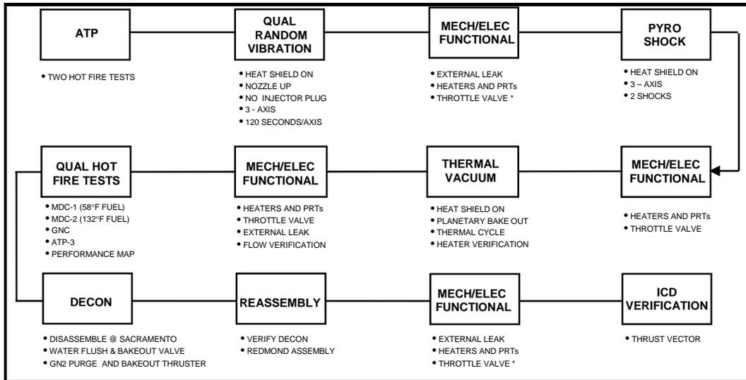
**Figure 4. Qualification Test Plan**
