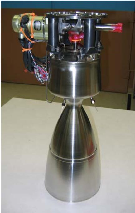
**Figure 10—MLE Engine with Nozzle Extension**
