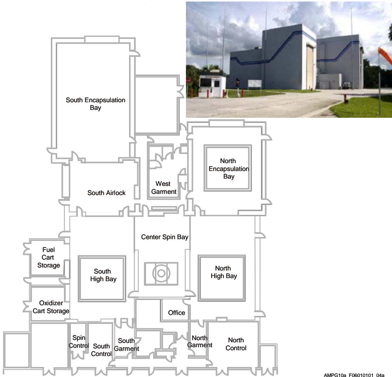
Figure 6.1.1.1-4 Astrotech Building 2 Hazardous Operations Facility
