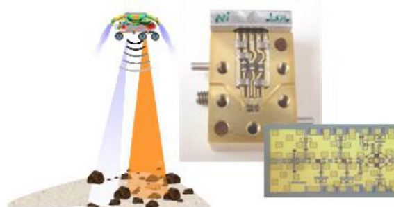
Figure10 – G-band radar for hazard detection, velocimetry, and altimetry
