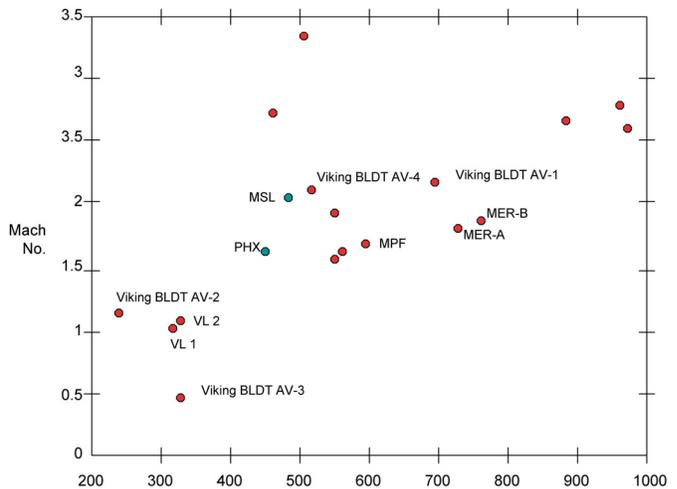
**Figure 13:** Mach and dynamic pressure history for all successful inflation disk gap band parachutes in Mars relevant conditions.
