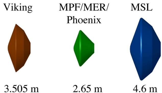
**Figure 10:** Viking-heritage 70-degree sphere-cone aeroshells.
