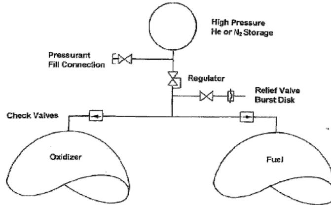
Note: Redundancy & Instrumentation Omitted
